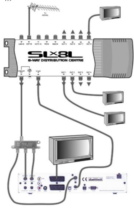
Note: the splitter feeding the various Toppy RF inputs can be omitted if the signal quality is high. Do this by using the two RF loopthoughs shown above in the basic connection diagram.
