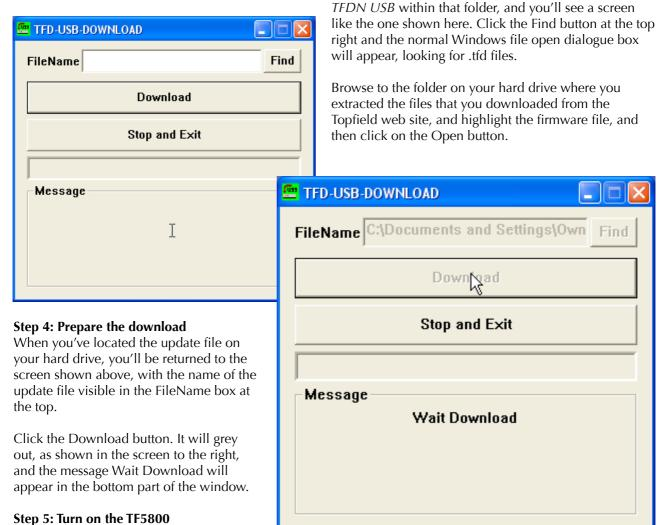
the firmware will be loaded from the PC via the USB port. With a USB 2.0 connection, the actual transfer time is around ten seconds.
